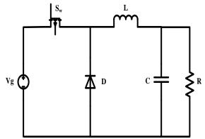
Fig. 5 DC-DC buck converter topology
