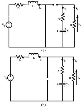
Fig. 8 Boost converter circuit (a) when switch is ON (b) when switch is OFF
