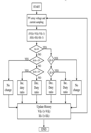
Fig. 9 Flow chart of the Incremental Conductance method
