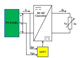
Fig. 1 DC-DC converter for operation at MPP
