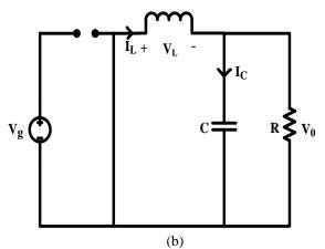
Fig.6 .Buck Converter Circuit when switch:- (a) turns ON (b) turns OFF
