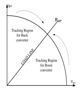
Fig. 10 Tracking of optimal resistance for Buck and Boost converter
