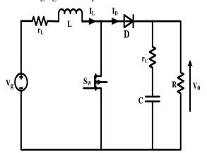
Fig. 7 DC-DC boost converter topology
