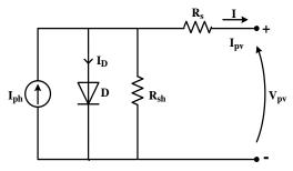
Fig. 2 Single diode model of PV cell
