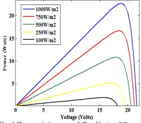
Fig. 4 Characteristics curve of (Ppv-Vpv) at different solar insolation
