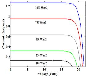
Fig. 3 Characteristic curve of (Ipv-Vpv) at different solar insolation
